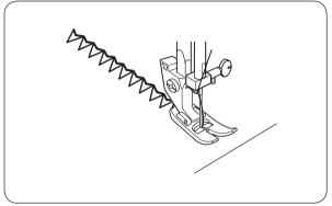
If forward and reverse feeds become unbalanced due to the type of fabric, adjust the balance by turning the stitch length dial as follows:
