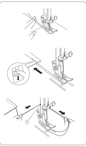
1 Raise the presser foot and position the fabric with its edge lining up with a seam guide line on the needle plate.
